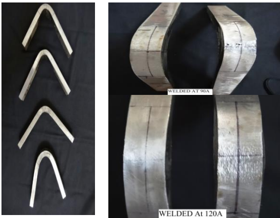
Fig. 8: Root bend test specimens at 90A and 120A
